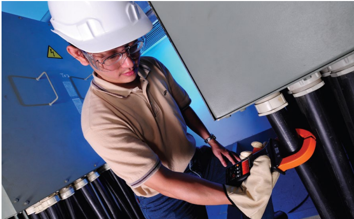
Figure 2. Large jaw clamp opening of 52mm / 2 inches
